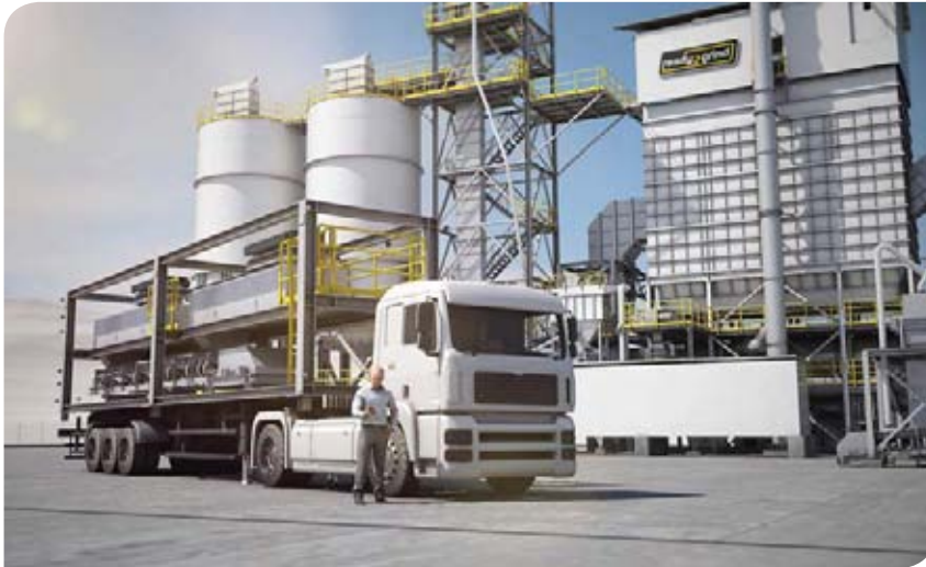
Above: The ready2grind system comes largely pre-assembled, resulting in lower installation times.
