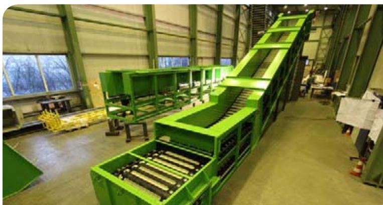
**Below:** Production of a surface feeder for unloading alternative fuels from trucks.
