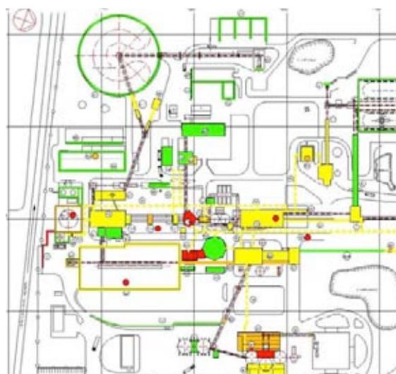
**Left - Figure 4:** Example of a plant layout showing the categorisation of the structures into risk classes.
