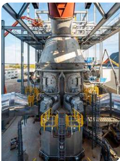
Below: The largest mill in Western Europe, an MVR 5300 C-6 in Belgium, is equipped with GPpro.
