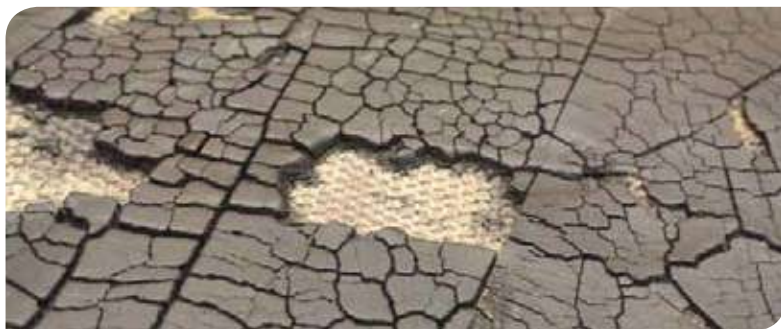
Above: Severe wear caused by heat damage that has been accelerated by UV exposure.
