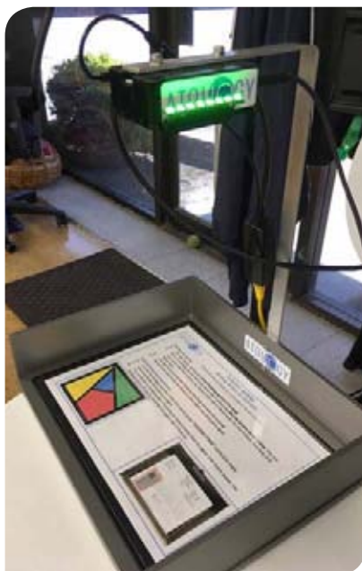
Below - Figure 2: An intelligent document holder that scans and irradiates the content placed in it.
