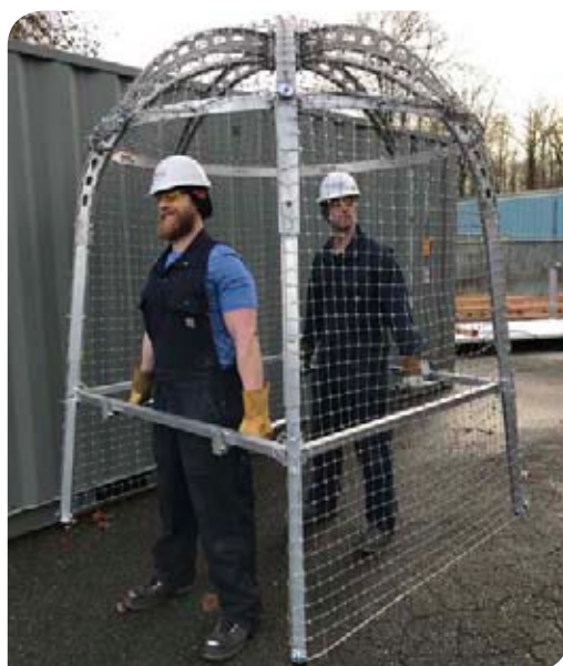
Right: Products manufactured with 6061-T6 aircraft aluminium offer an industry-leading strength-to-weight ratio. When used in safety cages, for example, this material is strong enough to protect workers from debris up to 140kg falling from a height of up to 2.4m, while still being light enough for two people to manoeuvre.
