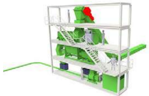
Above: Preparation and dosing tower with ODM-DiscSCREEN and ODM-WeighTUBE®.
