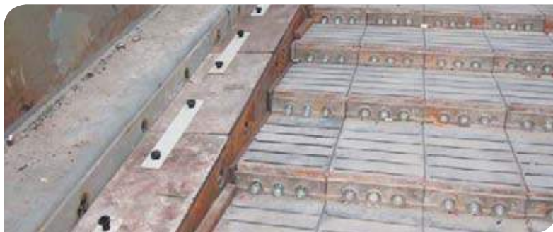
Above: A good example of minimised gaps on the grate.
