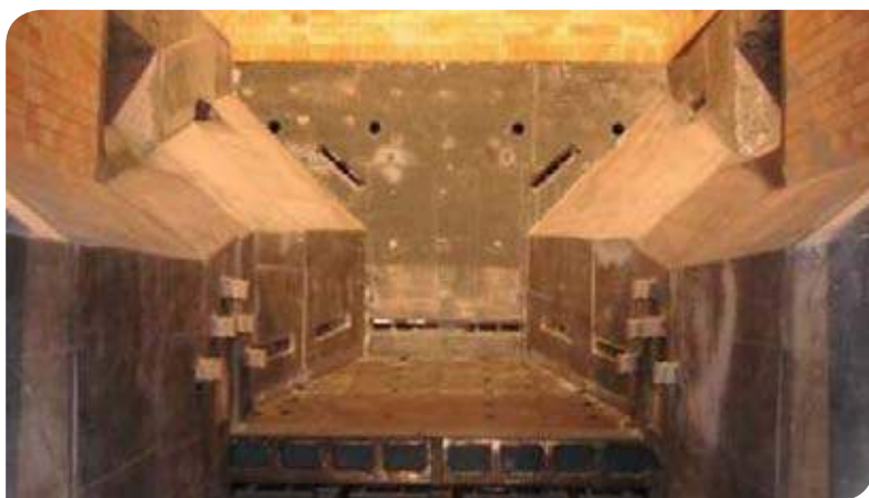
Below: The static inlet section is the most important part of the cooler.
