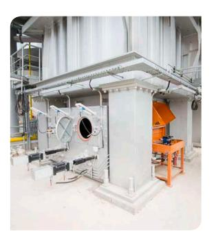
Left: The pulverised lignite is blown through burner lances into the kiln by AERZEN Delta Blowers. Source: www.sienk.de.
