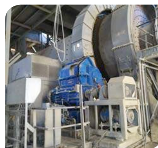
Above: A Lateral Gear Drive designed and manufactured by Wikov drives a horizontal ball mill at a cement plant in North Africa.
