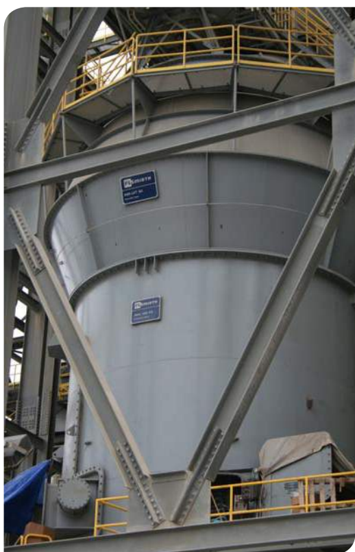
Above: There are six vertical roller mills at the Ste. Genevieve plant - two raw material mills and four finish mills. There are approximately 10 vertical roller mills presently used for cement grinding in the US. The image shows an FLSmidth Atox Mill vertical roller mill for raw material grinding.
