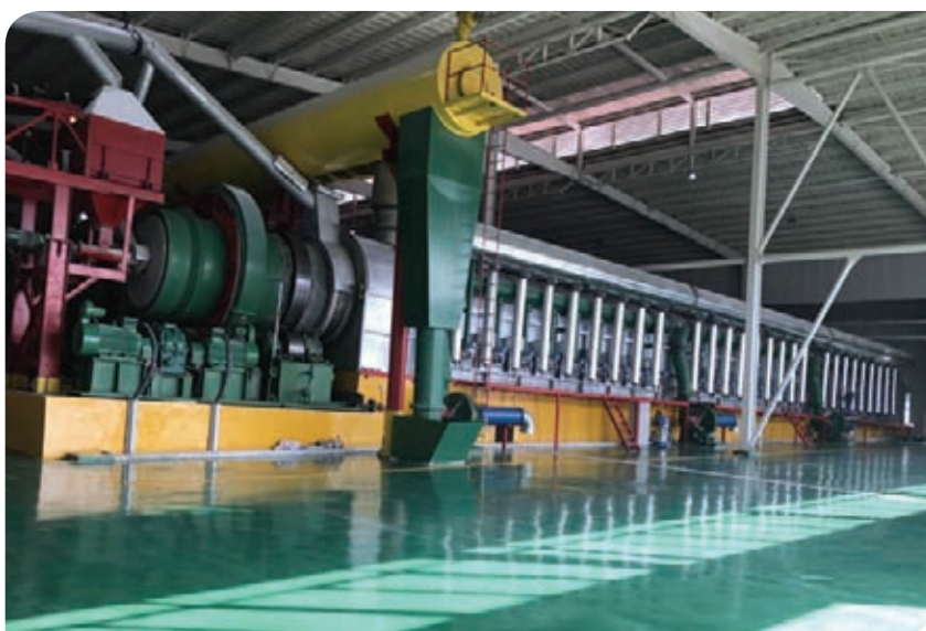
Below: One of four externally-heated rotary kilns that have been calcining magnesite on a demonstration basis since March 2018.
