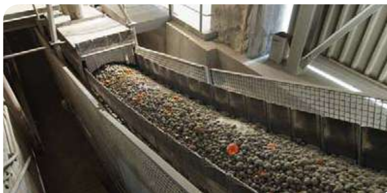
Above: An AUMUND KZB type Pan Conveyor handling hot clinker in a German cement plant.
