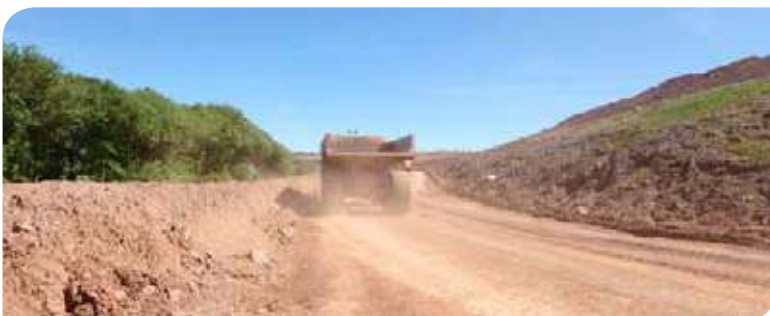
Below - Figure 3: An example of dust generation caused by a dump truck travelling along a haul road.
