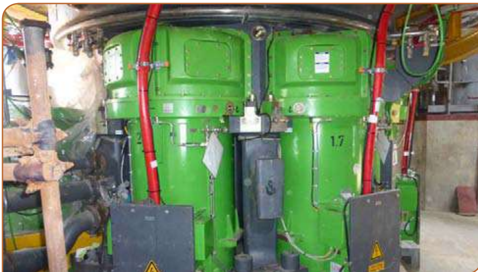
Above: The COPE drive from RENK can be linked to up to eight motors for ultimate redundancy.
