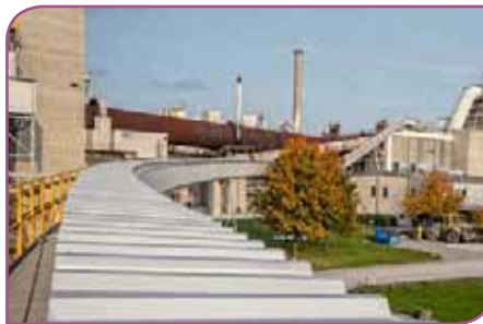
Top left - Figure 2: The feeding station of the Pipe Conveyor to the calciner. A take-up device has been installed at the rear. Source: BEUMER Group GmbH & Co. KG.
