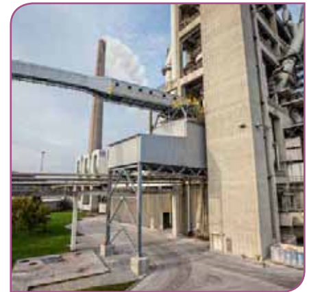
Top right - Figure 3: The two Pipe Conveyors: BEUMER Group realises different system solutions for the various bulk materials. Source: BEUMER Group GmbH & Co. KG.
