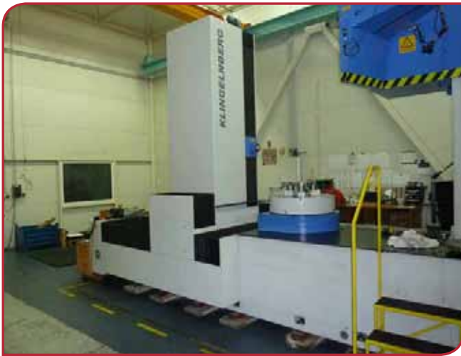
Above: Inspection of parts at Wikov Gear takes place in a climate-controlled environment at 20°C with a fixed humidity.
