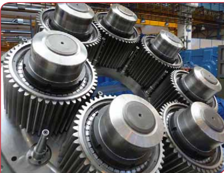
Below: Part of an Orbi-flex planetary gearbox originally commissioned for a large scale wind turbine.
