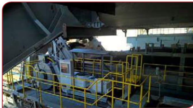
Left: Pilot low voltage GCD installation based on permanent magnet motors.
