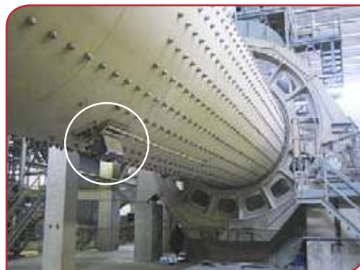
Right - Figure 1: An On Mill Unit (OMU) SmartFill (circled) on a two chamber mill. Level sensors for chamber 1 and chamber 2 are installed directly on the mill tube.
