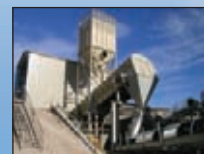
Truck Unloading Stations Receiving up to 1,200 t/h
