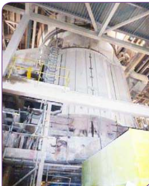
Left: The plant's large Polysius vertical roller mill for raw meal grinding.
