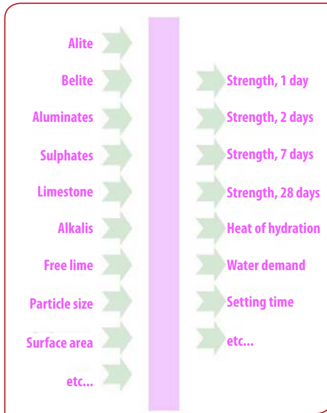
Right - Figure 2: A typical set of non-linear models for cement with composition and surface area as input variables.
