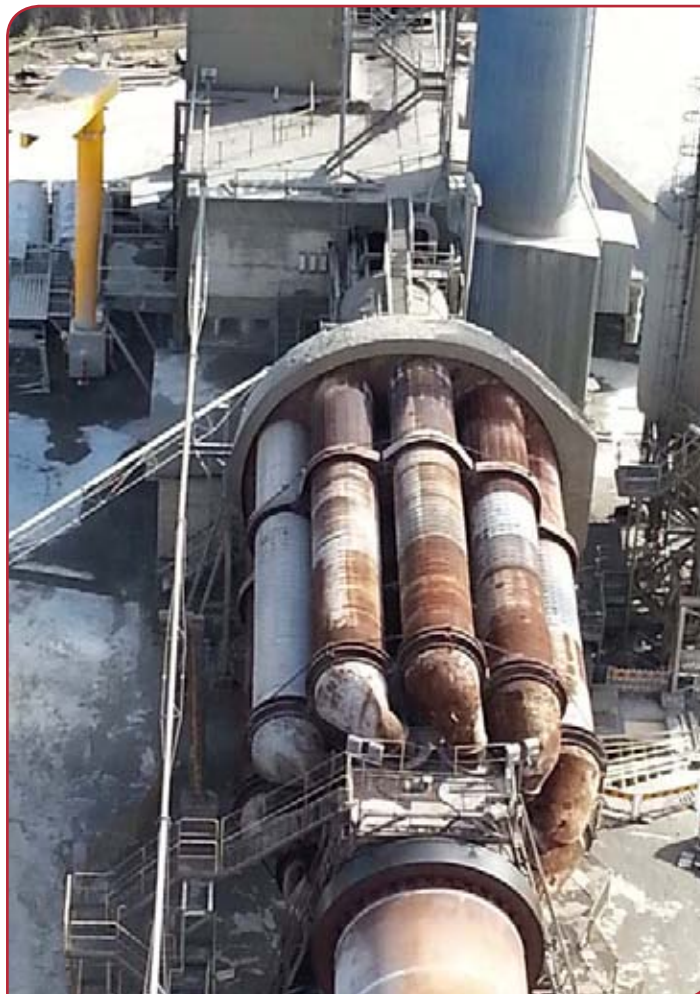
Right - Figure 1: Satellite coolers around the Finnsementti cement kiln in Pargas, Finland.
