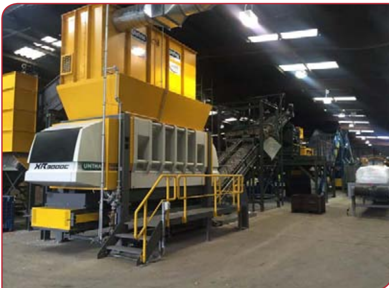
Below: A new UNTHA XR3000C shredder is at the heart of Avanti's new alternative fuel production process.
