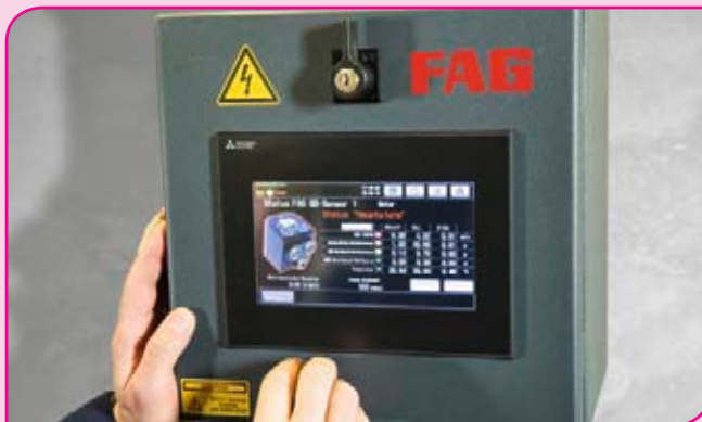
Above: The FAG SmartQB is a ready-to-use condition monitoring solution for electric motors, pumps and fans that is very easy to install and use.
