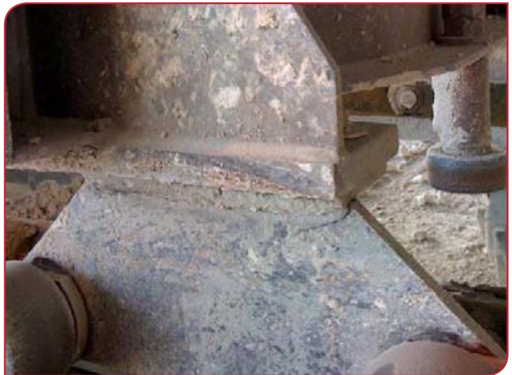
Above left - Figure 2: Damaged brushing on the original chain system.
