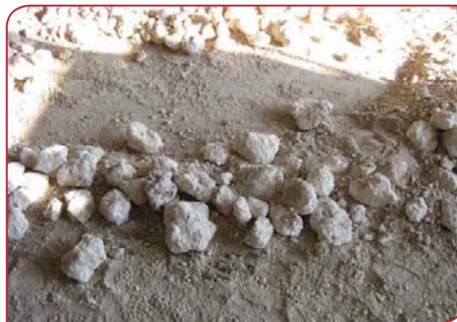
Right - Figure 1: Shock loads, which were being caused by large chunks of limestone, were damaging parts of the previous system.
