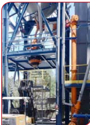
Below Right - Figure 3: The Flow Feeder uses pressure columns of material in a fluid state collected in the gravity chamber.
