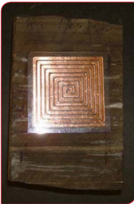
Above - Figure 1: Proof of concept sensor placed on a geological sample.
