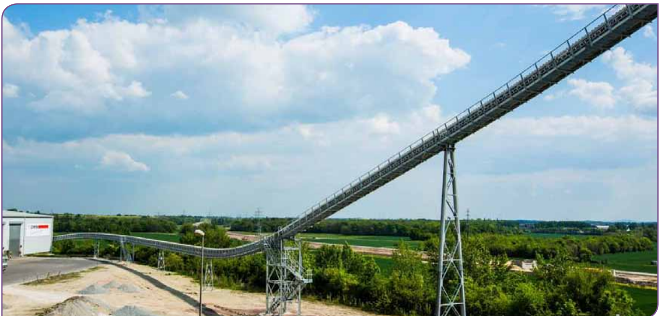
Below: Pipe conveyors can transport different types of bulk material over long distances, often through rough terrain.
