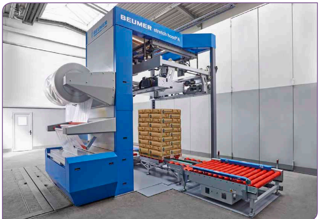
Right: The Beumer stretch hood covers the full pallets with a thin film hood. The bags arrive safely at their destination and the product is protected against humidity and atmospheric influences.
