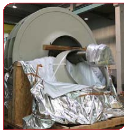
Far left: Peter Herrmann (General Manager Fans Division) and Inge Teich (Marketing) proudly stand next to a rotor for a filter fan for a customer in Colombia. Flow volume: 780,000m 3 /hr. Drive power: 2400kW.
