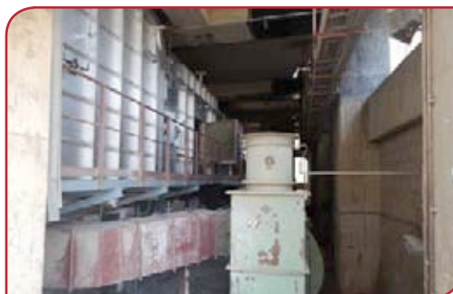
Left - Figure 3: An FLSmidth Cross Bar Cooler has replaced the old generation cooler.
