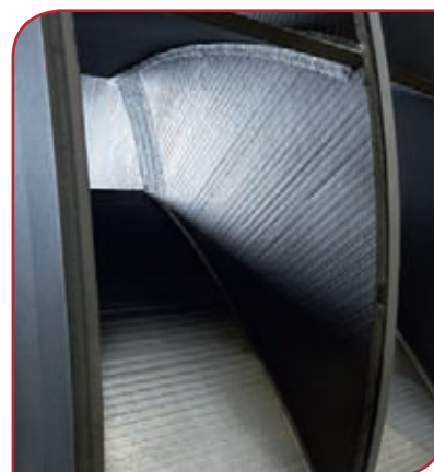
Left: Kiln fan impeller with special wear protection for a 10,000t/day cement production line in Saudi Arabia Impeller diameter: 3.4m. Drive power: 2800kW.
