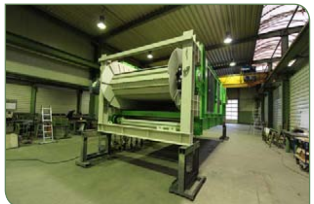
The apron conveyor, for raw material up to 200mm particle size, that DI MATTEO delivered to a cement plant client in North Africa.
