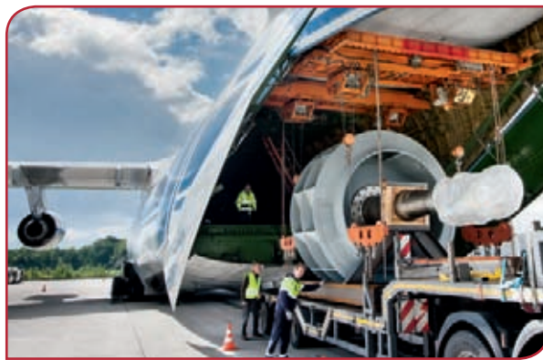
Left: Rotor for an exhaust air fan for an African cement company being specially despatched by Antonov. Flow volume: 1,600,000m 3 /hr. Impeller diameter: 3.46m. Rotor weight: 26,000kg.
