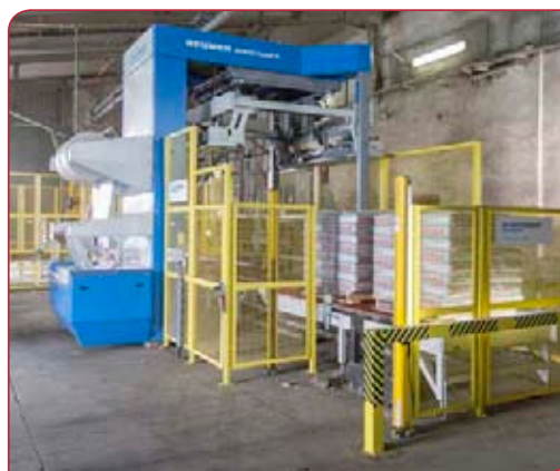
Left: The new BEUMER stretch hood A packaging system has a high packaging capacity at a low energy consumption rate.
