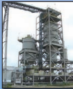
Silo Dischargers Discharging up to 1,000 t/h
