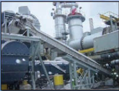
Chain Conveyors Conveying up to 1,000 t/h
