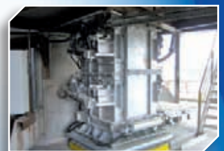
Secured double valve airlock with sliding gate
