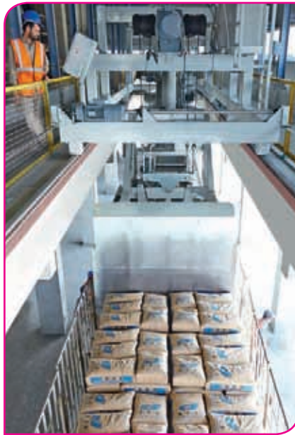
The HAVER Speedroad seen loading a truck from above..
