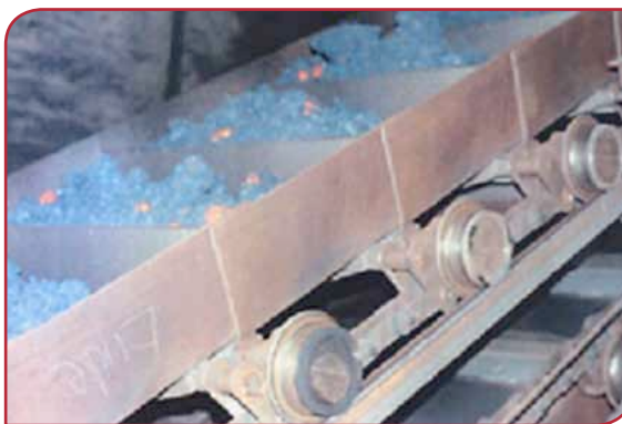
Left: Clinker coolers provide chains and their lubricants with a lot of challenges.
