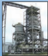
Silo Dischargers Discharging up to 1,000 t/h
