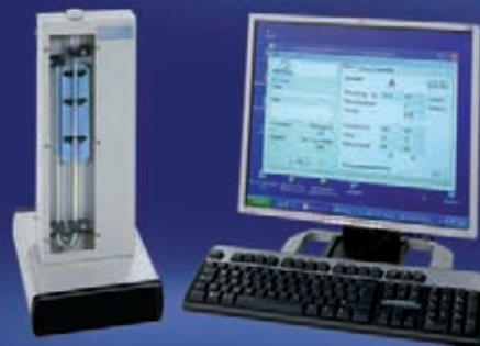
Blaine, PC operated, fully automatic
