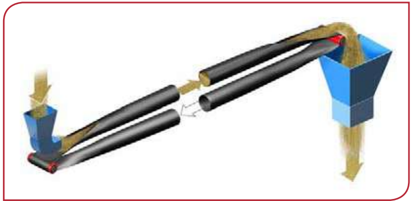
Above - Figure 3: The transport principle of the KOCH Pipe Conveyor.
