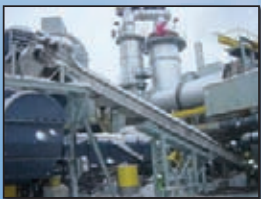
Chain Conveyors Conveying up to 1,000 t/h
