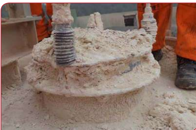
Below: Material in and around a PRV is a ‘tell-tale sign’ that something’s wrong.
