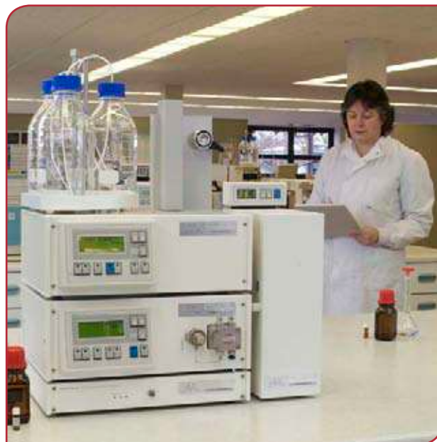
Right - Figure 1: A Cecil Instruments isocratic Adept high performance liquid chromatography (HPLC) system.
