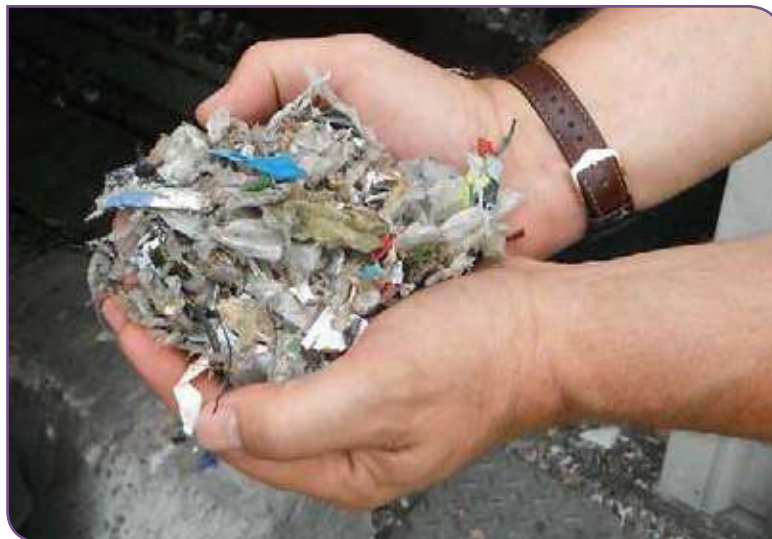
Right: Shredded, solid fuels derived from waste are used throughout the cement industry.
