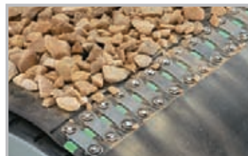
MECHANICAL BELT SPLICING
