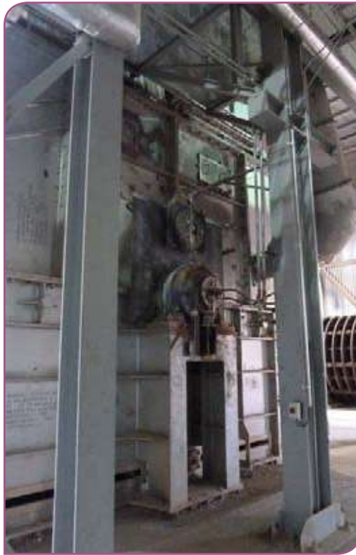
Right: The KHD raw meal grinding section is an unusual Tandem design. It comprises a 720t/hr dryer/crusher (left) and 360t/hr ball mill (right).
