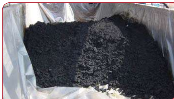
Below - Figure 5: Centrifuged WWT solids.
