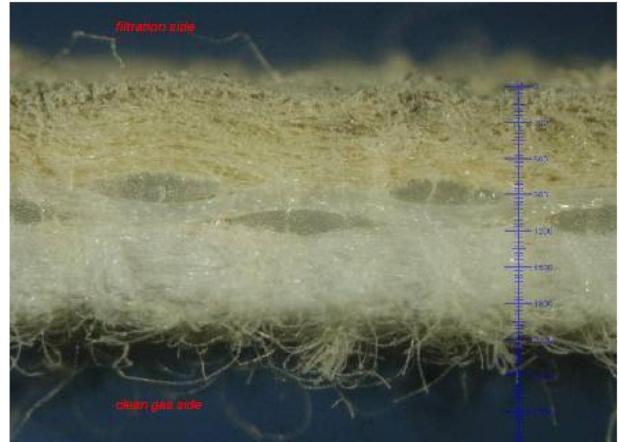
P84-PET fibre blend after 48 months
