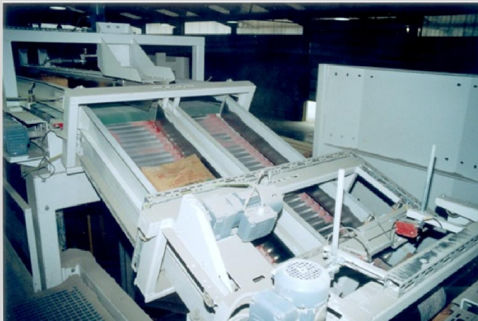
3rd step – roller conveyor
