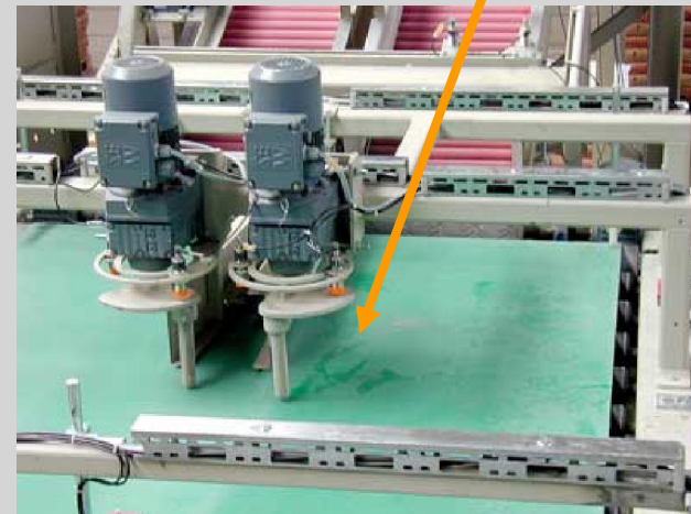
2nd step – bag turning device
