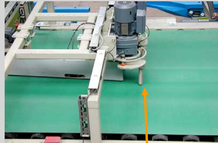
2nd step – bag turning device
