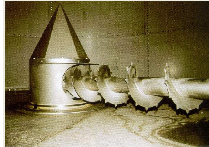
Aslan Cimento, OYAK Group, Turkey Silos with explosion venting and silo extraction screw
