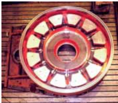
Figure 5: Segmented hydrodynamic/semi-hydrodynamic axial thrust bearing
