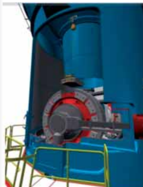
Figure 4: Segmented and 'oversize' rollers mean low risk of cracking, easy segment reversal and a coarser mill feed.
