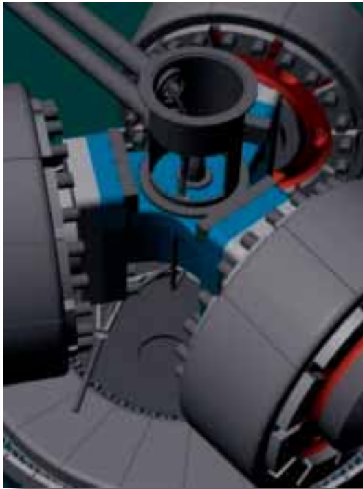
Figure 8: Water injection provided via the central part of the roller suspension system: water of previously-used water injection pipes is eliminated.
